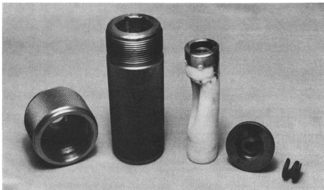
Fig. 14. A PTFE vessel after a pressure decomposition of an organic compound at 170^\circ\text{C} with a mixture of 0.2 ml of \text{HNO}_3 (70%) and 0.6 ml of \text{HClO}_4 (60%).
