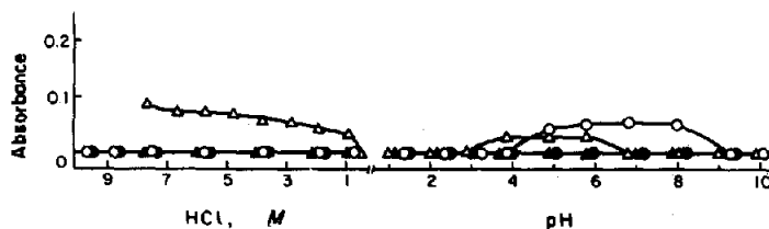
Fig. 3. Effect of acidity on the extraction of Te(IV) and Te(VI) with dithizone. O, Te(IV)-CCl 4 ; ●, Te(VI)-CCl 4 ; Δ, Te(IV)-MIBK; ▲, Te(VI)-MIBK; aqueous phase, 25 ml; organic phase, 10 ml; Te(IV) or Te(VI), 2 \mu g.
